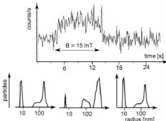
**Fig. 3:** Dependence of the distribution of cluster sizes on an applied magnetic field. Clusters which a diameter of about 1  $\mu$ m, formed in the magnetic field, decay in some seconds after turning-off the field.
