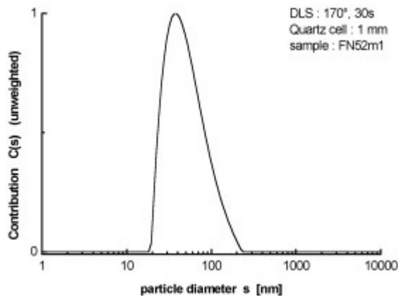
**Fig.2:** Particle size distribution of the pulse etched polycentric ferrofluid obtained by DLS of the concentrated original sample (back scattering, 170°).
