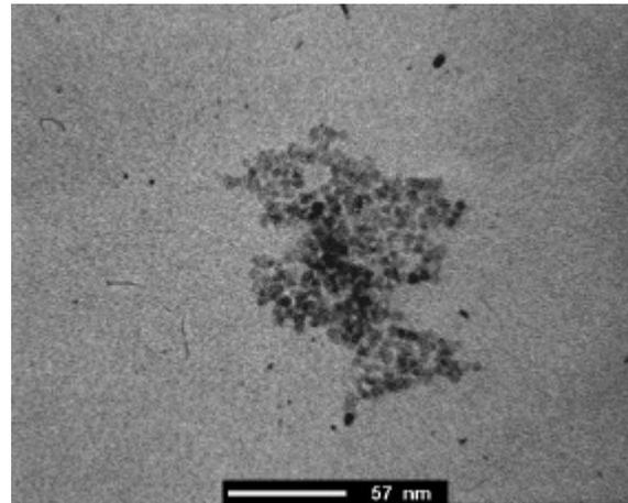
**Fig.3:** Structure of polycentric ferrofluid after shell exchange by phosphodextrane depicted by iron electron microscopy .
