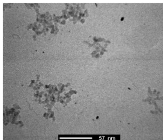
**Fig.1:** Structure of the pulse etched polycentric ferrofluid after size separation depicted by iron electron microscopy .
