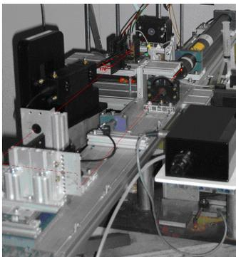
Dynamic Light Scattering device (DLS) at TUM-E17. The modular setup can be equipped with a magnet or stopped-flow device for field and time-resolved experiments. The backscattering setup (170°) enables the investigation of concentrated original samples (5 % w/w).
