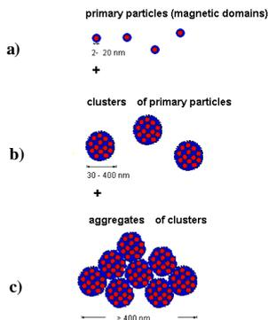
Due to EM and DLS investigations of several products, the hydrophilic shell Ferrofluids exhibit a three stage structure hierarchy:
