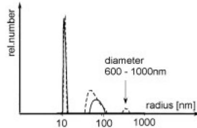
Dynamic light scattering of a Ferrofluid sample, sampling time are 3s (solid lines) and 1h (dashed lines). The large particles are difficult to detect (long time only), due to the small active volume.
