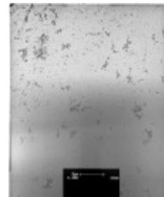
**Overview** image of a commercial hydrophilic shell Ferrofluid with attached drug (Mitoxantrone) obtained by direct Electron Microscopy. The sample consists of three types of nanoparticles: single domains, clusters and aggregates of clusters.
