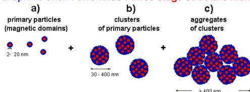
Due to EM and DLS investigations of several products, the hydrophilic Ferrofluids exhibit a **three stage structure hierarchy** [2]:
