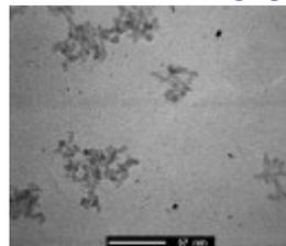
**Structure** of the pulse etched polycentric Ferrofluid after size separation depicted by **electron microscopy** (iron image) [2].
