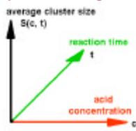
The **Ferrofluid cluster size**  $S(c, t)$  depends on reaction time  $t$  and acid concentration  $c$  during **pulse etching**.
