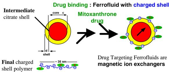
**Ferrofluid shell exchange:** Ferrofluid-clusters of medium size (50-100 nm diameter) are embedded by citrate and negatively charged **phosphodextrane** (10kD), after synthesis with an intermediate citrate shell
