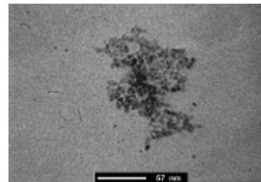
**Structure** of a polycentric Ferrofluid after **shell exchange** by **phosphodextrane** depicted by iron electron microscopy (no stain, O. Stroh, diploma thesis, TU München in prep.).
