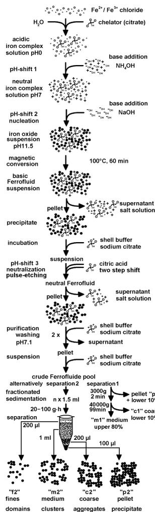
**Synthesis flow chart** of biocompatible Ferrofluid, size control by **pulse etching** and **separation by sedimentation** [2].
