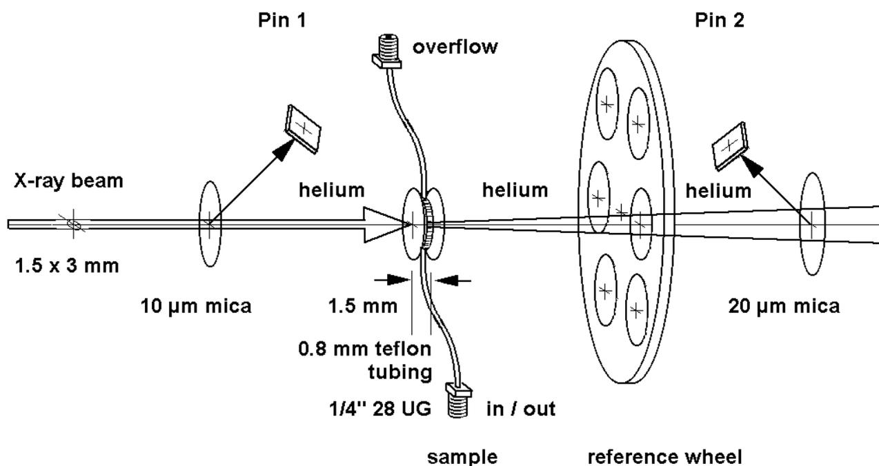
Figure 1: Sample environment for SAXS with protein or polymer solutions in a flat mica flow-through cell.
