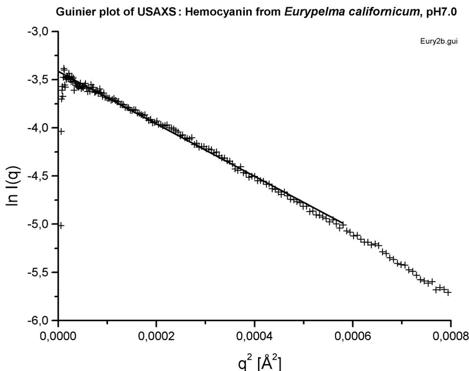
Figure 1: The Guinier representation of USAXS of Hemocyanin from *Eurypelma californicum* (10g/l) yields at pH7.0 an apparent radius of gyration of  $R_g = 90.31 \pm 0.31 \text{ \AA}$  ( $q$  (fit) =  $0.00336 - 0.0225 \text{ \AA}^{-1}$ ).
