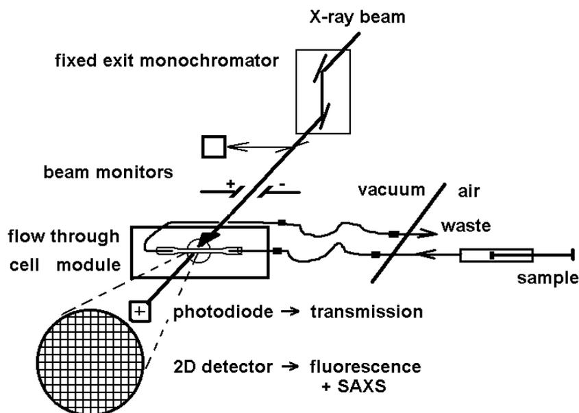
Figure 1: Setup for XANES, EXAFS and ASAXS of metalloprotein solutions with a flow through cell at the JUSIFA beamline (B1). The stable quartz capillary allows the estimation of true reference spectra.
