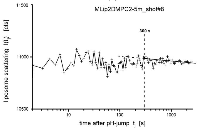
**Fig.3)** During time resolved neutron scattering of liposomes from DMPC (10g/l, H<sub>2</sub>O) after a strong pH-jump to pH13 by stopped-flow mixing (1:1) with 0.5 M NaOH-KCl buffer the iron oxide deposits within 220s, the liposomes decompose after  $t_j > 600s$ .; while **(Fig.4)** after a moderate pH-jump to pH11.5 with 0.05 M NaOH- buffer, the liposomes are stable for  $> 2000s$ , the iron oxide shell deposits during 300 s.
