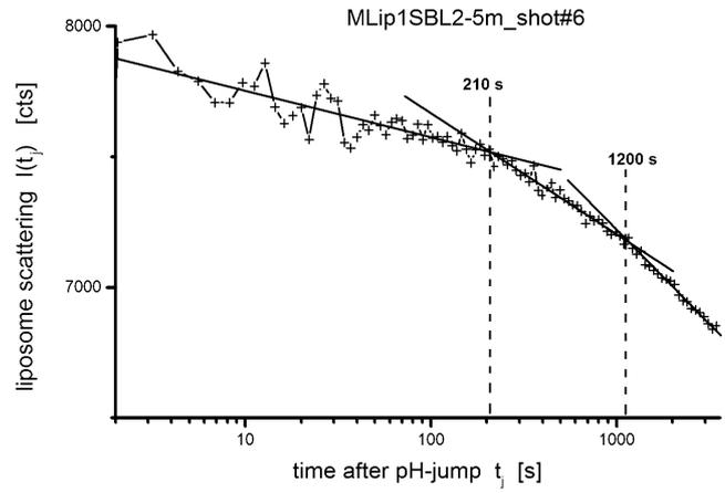
**Fig.1)** During time resolved neutron scattering of liposomes from SBL (10g/l, H<sub>2</sub>O) after a moderate pH-jump to pH10.5 by stopped-flow mixing (1:1) with 1 M Tris-KCl buffer the iron oxide deposition takes 1300s, the liposomes decompose after 1h (4000s); while **(Fig.2)** after a large pH-jump to pH13 with 0.5M NaOH-buffer, decomposition starts at 210-1200s.
